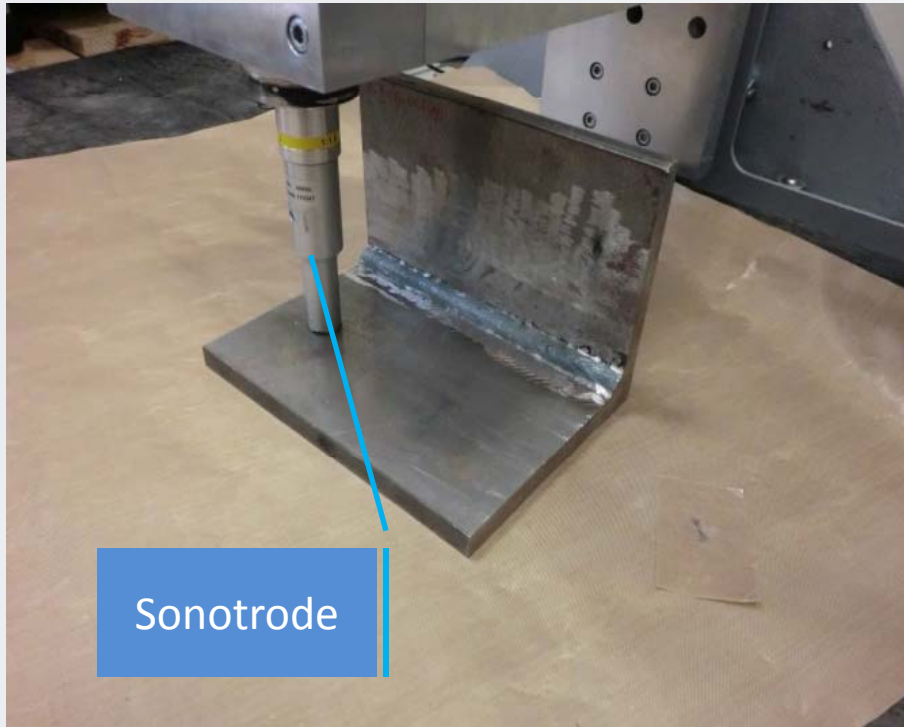
Weld test specimens – cold laps in weld
