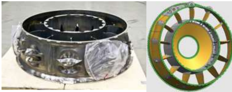
TEC (Turbine Exhaust Case)– Ni based alloy
