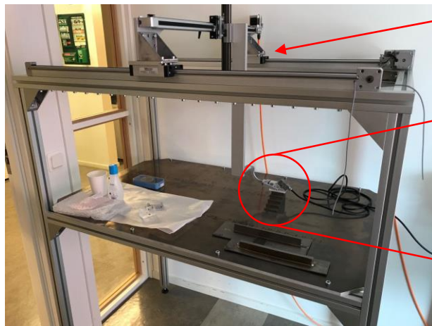
Mechanized gantry system
